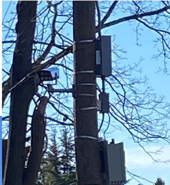
Fixed LPR / Fixed LPR2 / Mobile LPR - License plate readers, whether fixed or mobile, can be a cornerstone technology in RTCCs, constantly monitoring for wanted and stolen vehicles.
