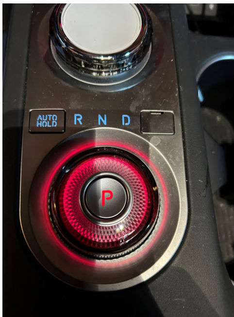
Genesis – A rotary computer-controlled transmission selector.
